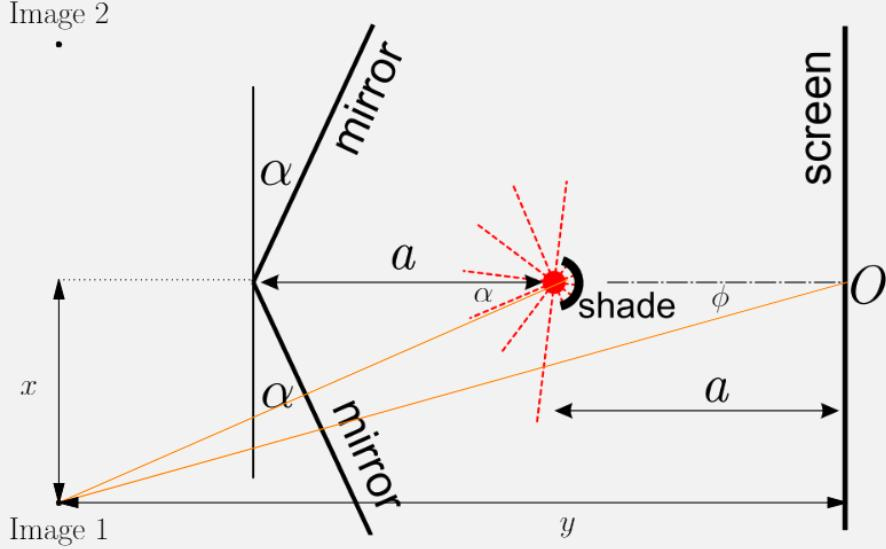
We find light source images in mirrors. The light incident around  $O$  can then be viewed as a superposition of the light emitted from the images. We first find  $\sin \phi$ .
